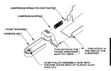
Figure 5-6. Installation of Frame Tensioner.
